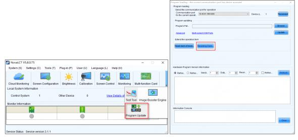
Access 2: Screen Configuration > Receiving Card > Program Update > Receiving Card Cloud Update. This entry automatically matches the chips shown in the receiving card interface.
