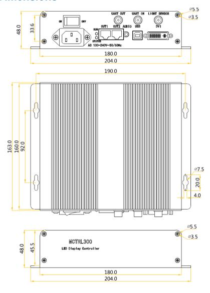
Tolerance: ±0.3 Unit: mm
