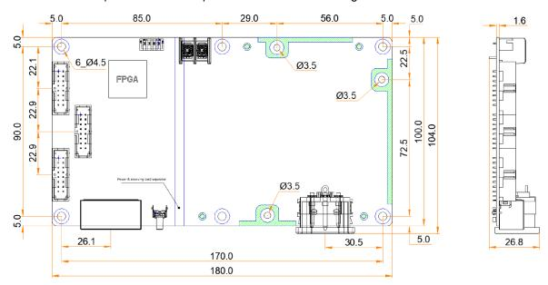
Tolerance: ±0.3 Unit: mm
