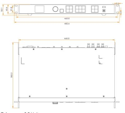
Tolerance: ±0.5 Unit: mm
