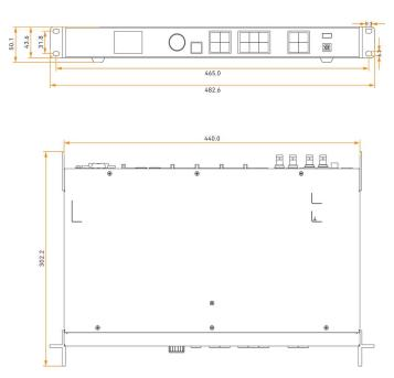
Tolerance: ±0.5 Unit: mm
