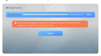
Press the left/right button to increase or decrease the screen brightness. After adjustments, press the direction button to select **Save** and press the OK button to automatically save the brightness parameter.
