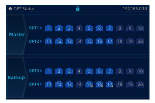
• When a PIXELHUE video processor is connected to OPT 1/OPT 2, the port is used an input connector. The OPT status page displays the resolution and frame rate of the accessed OPT source and the connection and backup statuses of the Ethernet ports on the fiber converter connected to the VX2000 Pro, as shown in Figure 4-3.
