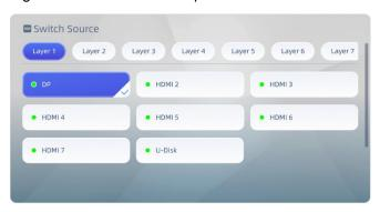
Press the direction button to select the desired layer and input source respectively. After selection, press the OK button to switch the input source of the selected layer.
