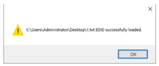
Step 10 Go back to **Workstation > View system topology** to check the EDID status. If the original **EDID** (**Monitor**) changes to **EDID** (**File**), the EDID is loaded successfully.
