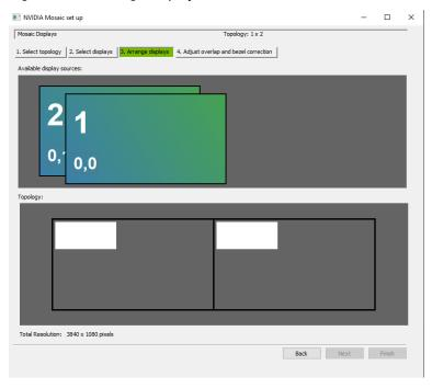
Step 10 Arrange the displays according to the screen arrangement and structure by dragging the available displays to the corresponding topology areas.
