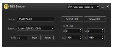
Step 2 Set the position and size of the screen on the computer to be used as NDI.
