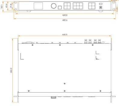
Tolerance: ±0.5 Unit: mm
