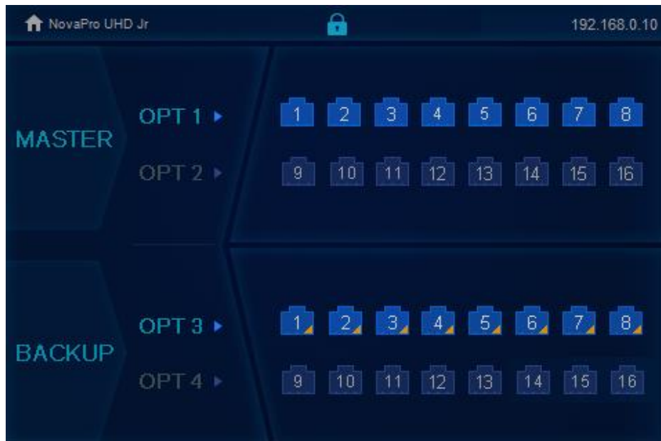
Figure 4-3 Optical fiber port statuses – Hot backup
