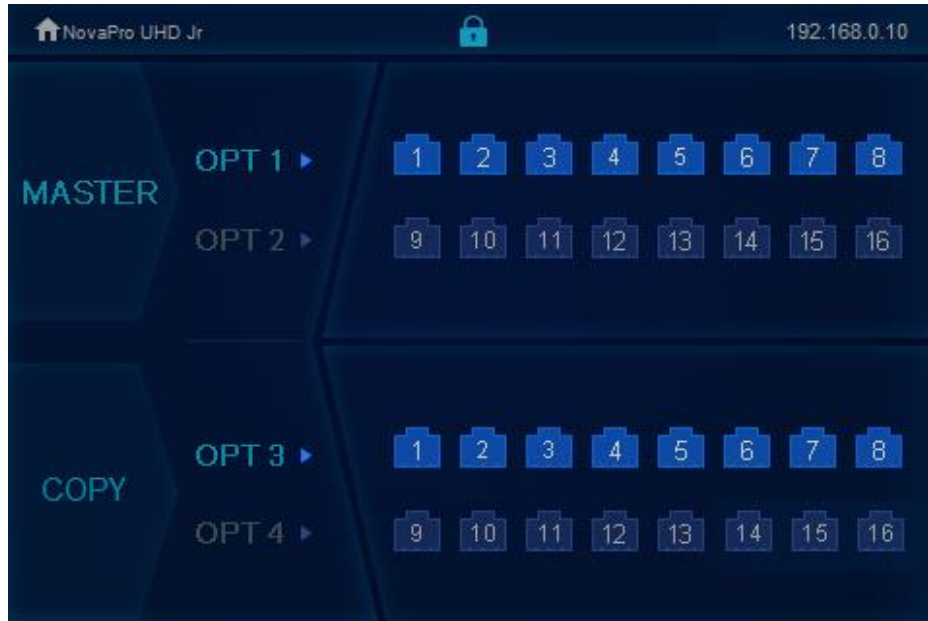
Figure 4-2 Optical fiber port statuses – Copy
