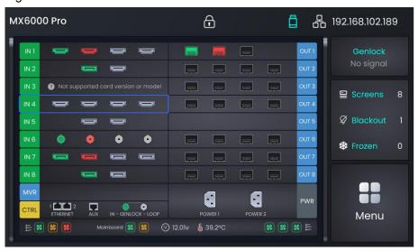
Figure 4-2 Input and output card details
