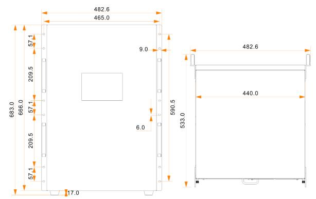
Tolerance: ±0.5 Unit: mm
