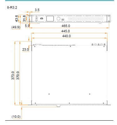
Tolerance: ±0.3 Unit: mm
