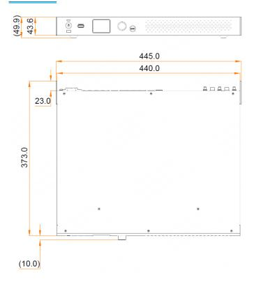
Tolerance: ±0.3 Unit: mm
