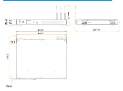
Tolerance: ±0.3 Unit: mm
