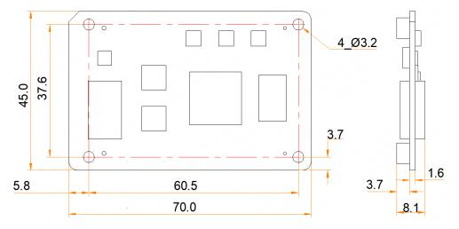
Tolerance: ±0.3 Unit: mm
