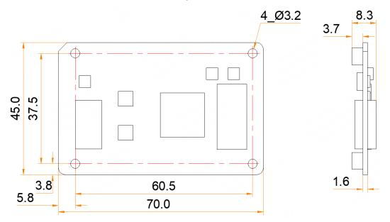
Tolerance: ±0.3 Unit: mm
