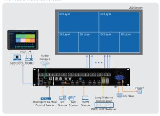
• Work as a fiber converter for long distance transmission
