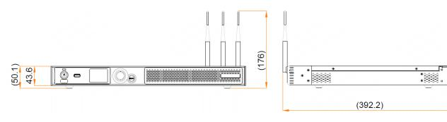
Tolerance: ±0.3 Unit: mm
