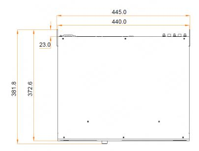
Tolerance: ±0.3 Unit: mm
