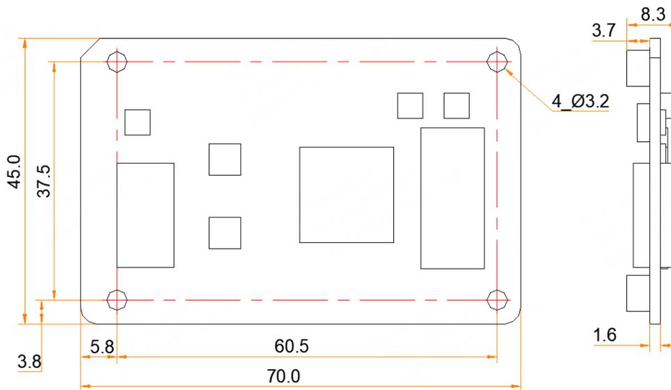
Tolerance:  $\pm 0.3$  Unit: mm
