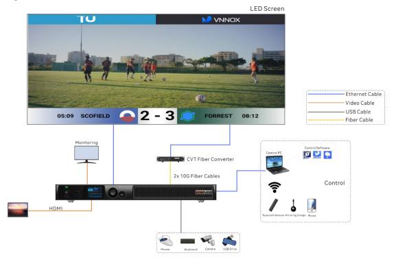
Step 4 Connect the Ethernet cables from the LED screen to the Ethernet output ports of TU4K Pro in the order shown below.
