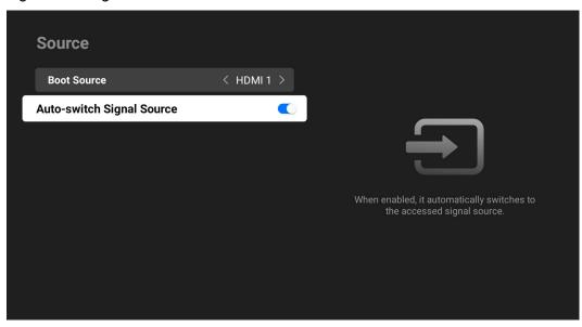
Step 3 Select a **Boot Source** option from the following: **Android**, **HDMI 1**, and **HDMI 2**. Press the left and right buttons to switch between the signal sources.
