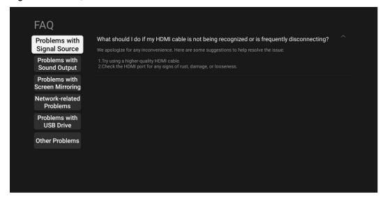
Step 2 Use the remote's **Up** and **Down** buttons to toggle between the categories of issues on the left, then press the **Confirm** button to view the specific questions.
