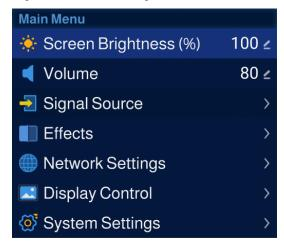
Step 2 Rotate the knob to adjust the brightness to the desired level and then press the knob to complete the adjustment.
