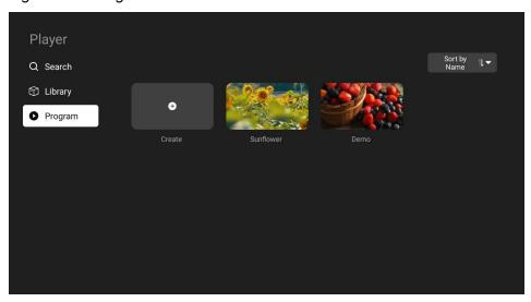
Step 3 To create a new program, select **Create**, select the desired media files from the library and then press the **Confirm** button on the remote.
