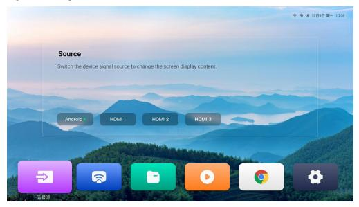
Step 2 Select the signal source that you want to display, and press the **Confirm** button on the remote.
