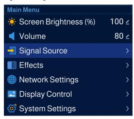
Step 2 Select a signal source (Android, HDMI 1, HDMI 2 or HDMI 3). Press the knob after a signal source is selected.
