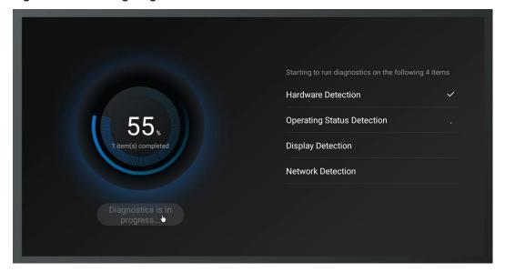
Step 3 Once the diagnostic process is complete, you will see either **Device normal** or **Device**abnormal displayed on the left. On the right, you can view the test items categorized as Normal, Abnormal, or Not tested. To see detailed information about all detected items, select View Report.
