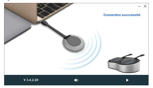
Step 3 When a pop-up window with the "Connection successful" message appears, press the round button on the dongle to start mirroring.
