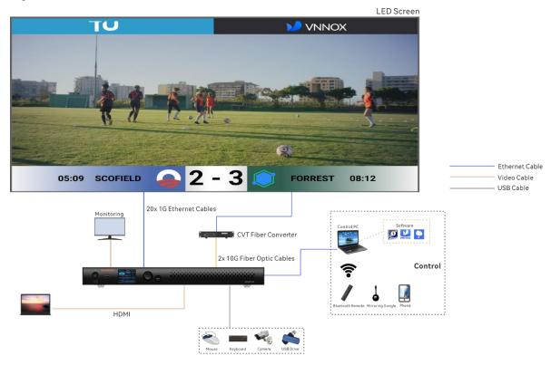
Step 4 Connect the Ethernet cables from the LED screen to the Ethernet output ports of TU40 Pro in the order shown below.
