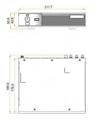
Tolerance: ±0.3 Unit: mm
