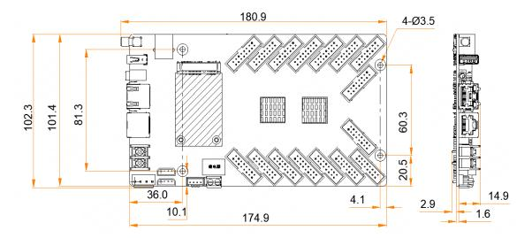
Tolerance: ±0.3 Unit: mm
