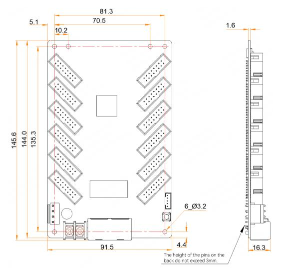
Tolerance: ±0.3 Unit: mm
