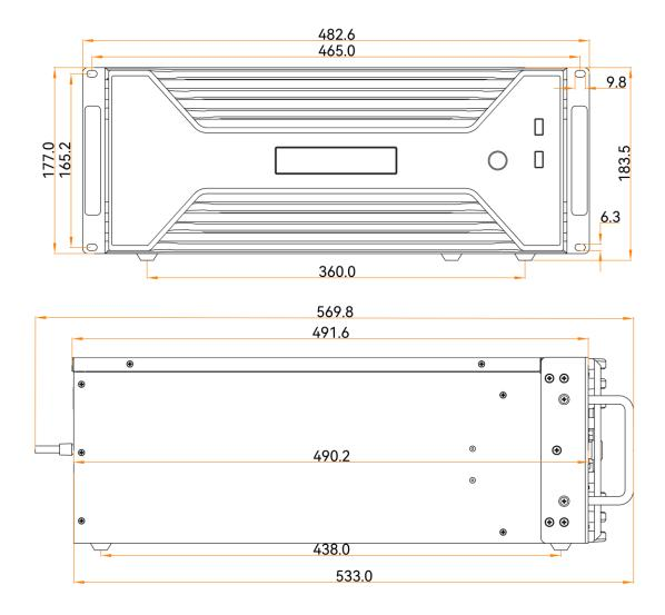
Tolerance: ±1 Unit: mm
