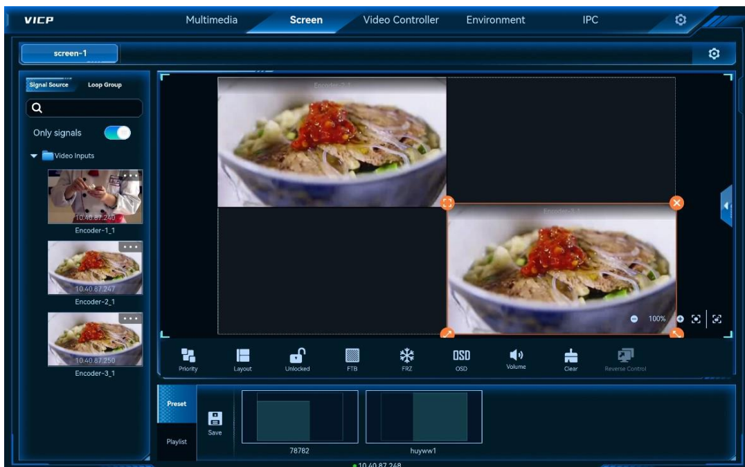
Figure 6-24 Input source switched successfully
