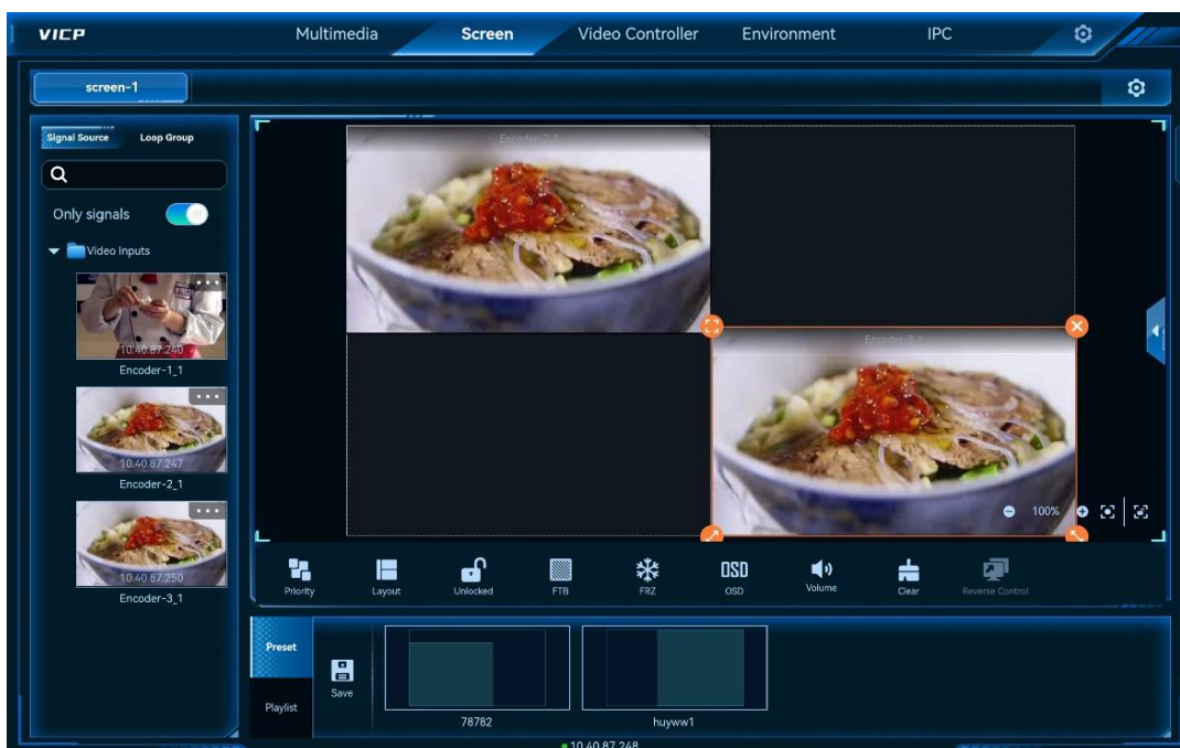
Figure 5-25 Input source switched successfully
