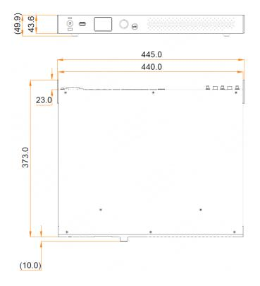
Tolerance: ±0.3 Unit: mm
