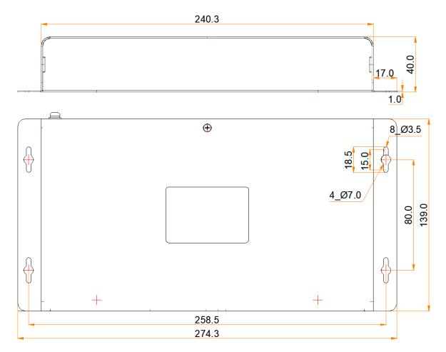
Tolerance: ±0.3 Unit: mm
