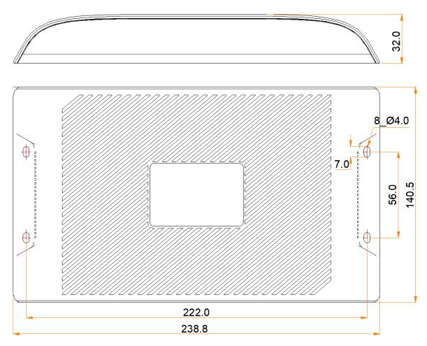
Tolerance: ±0.3 Unit: mm
