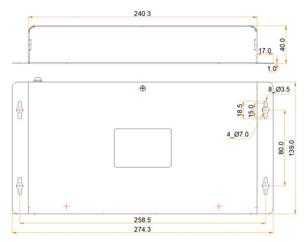
Tolerance: ±0.3 Unit: mm
