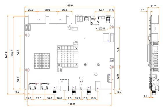
Tolerance: ±0.3 Unit: mm
