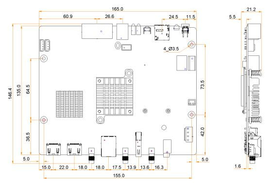
Tolerance: ±0.3 Unit: mm
