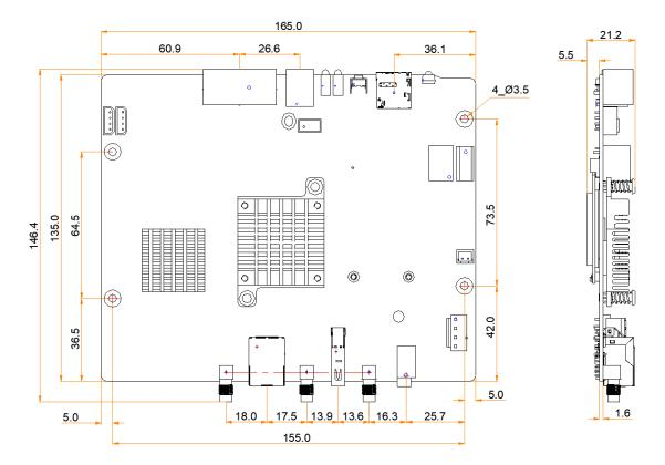
Tolerance: ±0.3 Unit: mm
