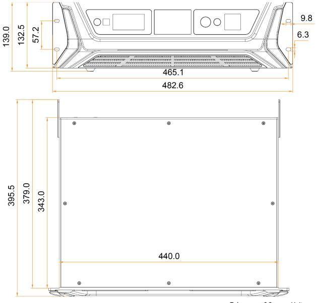
Tolerance: ±0.3 Unit: mm
