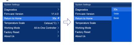
Step 2 Select 30s, 1min or 5min from the drop-down options as required.
