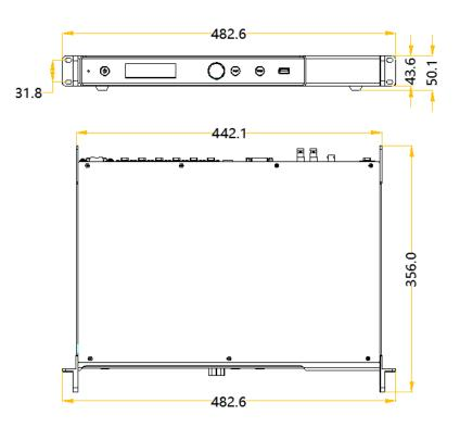
Tolerance: ±0.3 Unit: mm
