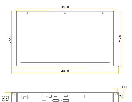
Tolerance: ±0.3 Unit: mm
