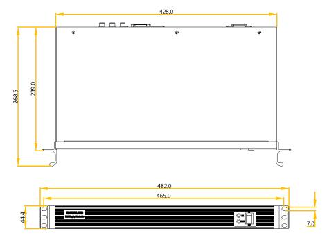
Tolerance:  $\pm 0.3$  Unit: mm
