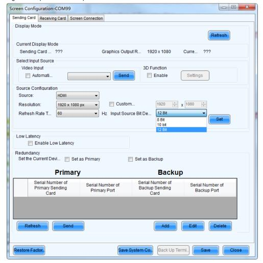
Table 7-1 Input source bit depth adjustment
