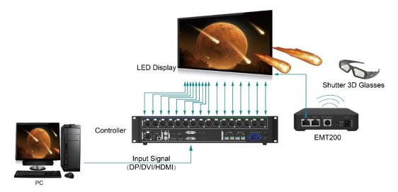
Application 2: EMT200 connected between the controller and receiving card
