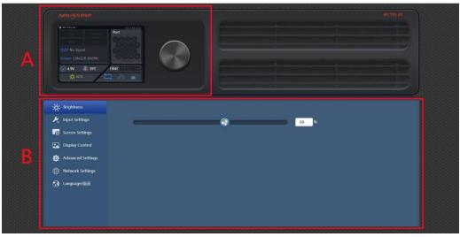
Area A: Hardware connection statuses and loading capacities of the input, output and other connectors on the MCTRL4K. For details, see chapter 5 Home Screen.
