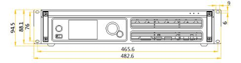
Tolerance: ±0.3 Unit: mm
