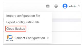
Step 3 After the backup is done, data such as source parameters, screen configuration files, brightness configuration parameters, and monitoring configuration parameters will be backed up to VNNOX Care cloud platform.
