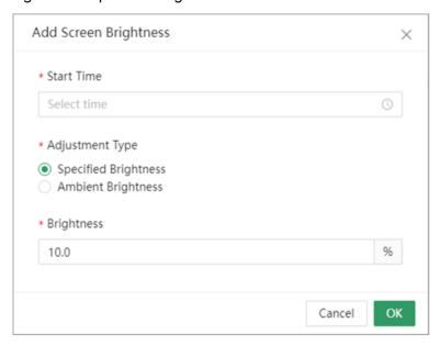
• Select **Ambient Brightness** and click **OK.** (This feature is available only when a light sensor is connected to the device.)
