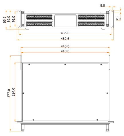
Tolerance: ±0.3 Unit: mm
