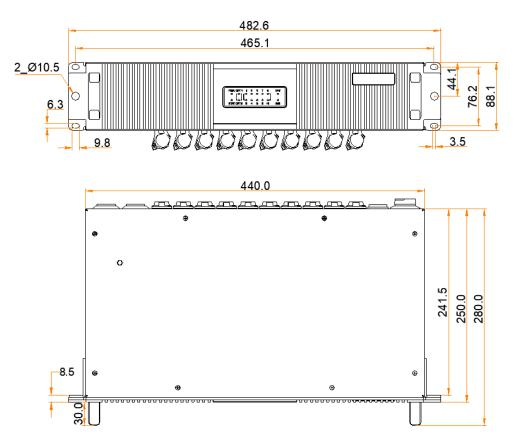
Tolerance: ±0.3 Unit: mm
