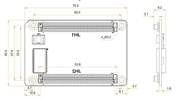
Tolerance: ±0.3 Unit: mm
