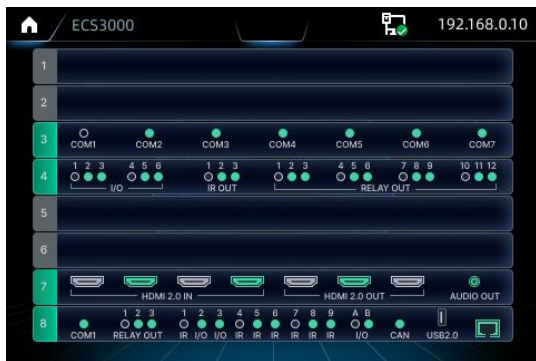
Figure 2-2 Backplane connector status
