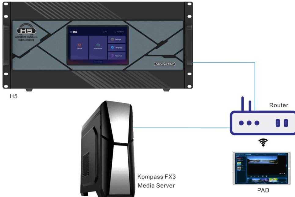
Figure 7-5 Connections for App control
