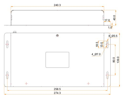
Tolerance: ±0.3 Unit: mm
