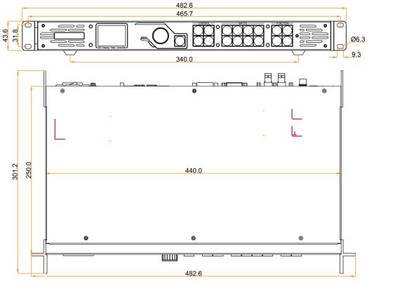
Tolerance: ±0.3 Unit: mm
