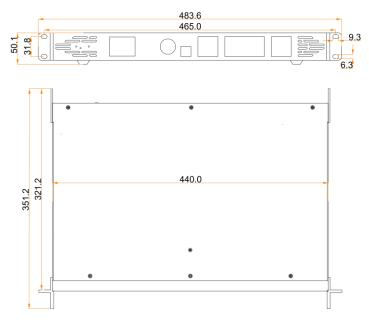
Tolerance: ±0.3 Unit: mm
