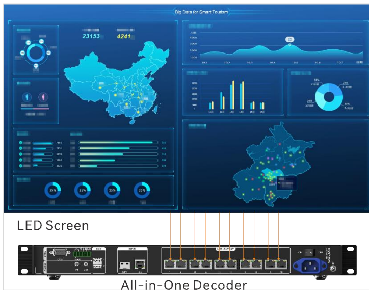
Figure 2-8 LED screen connections
