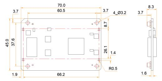
Tolerance: ±0.3 Unit: mm
