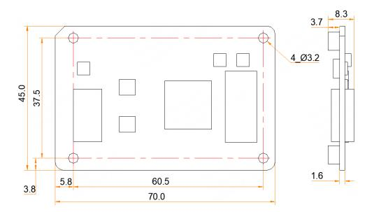
Tolerance: ±0.3 Unit: mm
